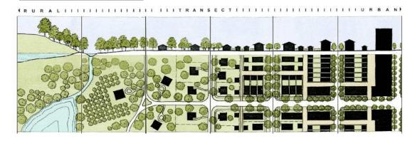
This diagram illustrates how the transect classifies elements of the human environment from rural to urban, in a left-to-right sequence. (Source: Duany, Plater-Zyberk, 2007)
